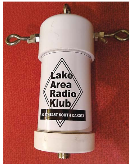
Figure 3 —The antenna connection on the outside of LARK's balun.
